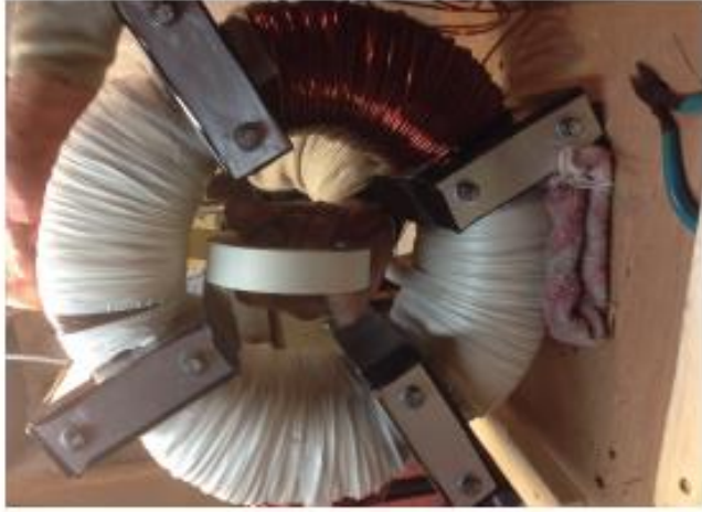
Installing outer wrap on core
