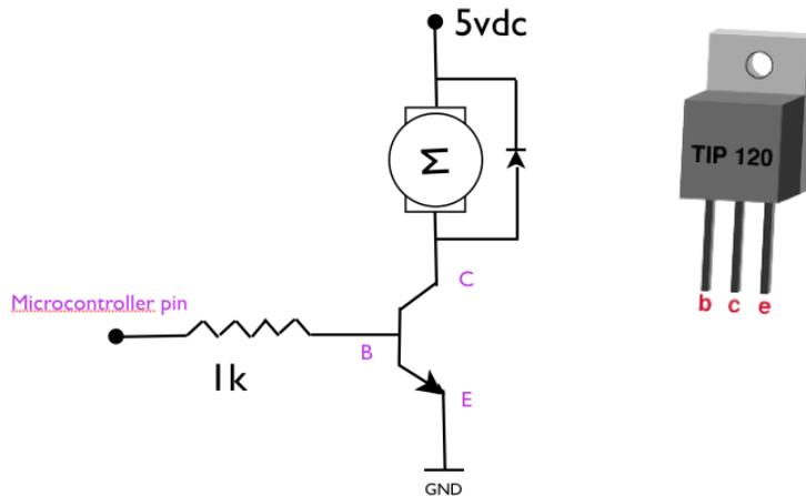
(yes i realize that the TIP120 is a Darlington pair and the above schematic shows a single NPN transistor. i found the image on the net, and as a "black box" it illustrates the configuration.)
