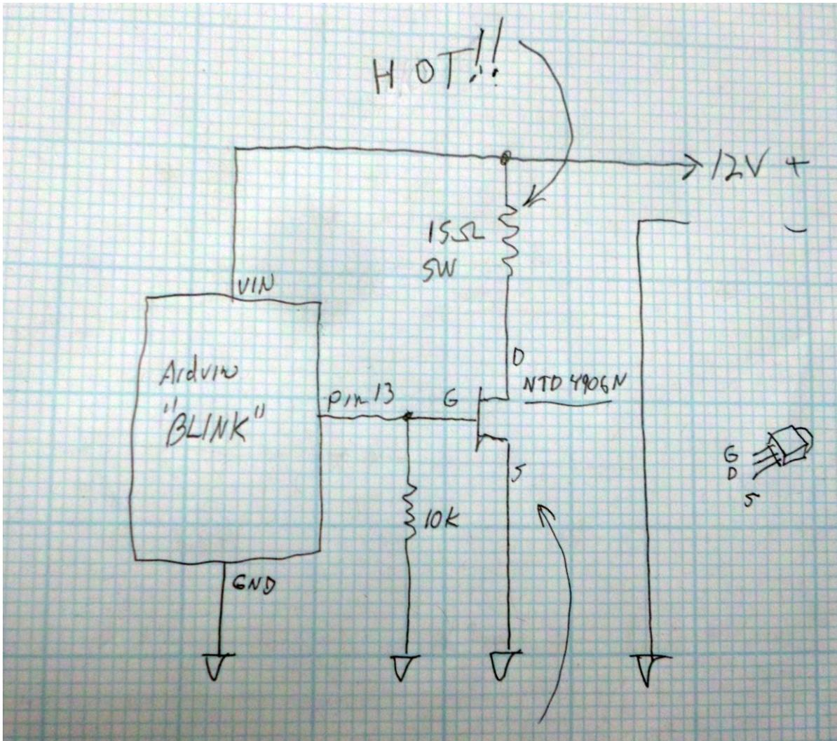
in this example i used a 15-ohm resistor, all i had to get the desired current range. just substitute your load in place of that resistor.
