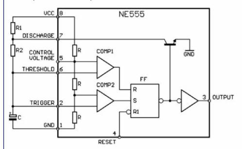
A capacitor C is charged thru a well known resistor array R1 + R2 until it's voltage reaches 2/3 of supply voltage. Then capacitor C is discharged by well known resistor R2 until capacitor voltage is 1/3 of supply voltage. then C is recharged again.
