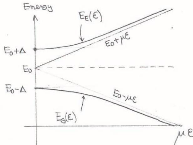
Figure 5: The energy levels of the two states of the ammonia molecule as a function of the magnitude  $\mathcal{E}$  of electric field. The higher energy state, with energy  $E_E(\mathcal{E})$  coincides with  $|E\rangle$  when  $\mathcal{E} = 0$ . The the lower energy state, with energy  $E_G(\mathcal{E})$  coincides with  $|G\rangle$  when  $\mathcal{E} = 0$ .
