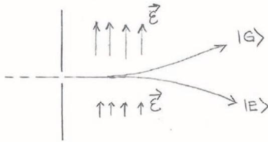
Figure 6: If a beam of ammonia molecules is exposed to an electric field with a strong gradient, molecules in the ground state  $|G\rangle$  are deflected towards the stronger field (up) while molecules in the excited state  $|E\rangle$  are deflected towards the weaker field (down).
