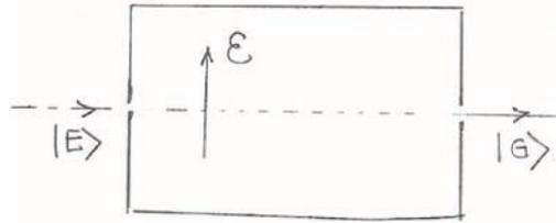
Figure 7: A resonant cavity tuned for 23.87GHz. A beam of ammonia molecules in the excited state  $|E\rangle$  enter from the left. If properly designed, the molecules exit the cavity from the right on the ground state  $|G\rangle$ . In this process each molecule adds energy  $2\Delta$  to the electromagnetic field in the cavity.
