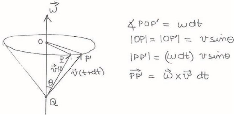
Figure 1: The vector  $\mathbf{v}(t)$  and an instant later the vector  $\mathbf{v}(t + dt)$ . The angular velocity vector  $\boldsymbol{\omega}$  is along the axis and  $\mathbf{v}$  rotates about it with origin  $Q$ . At all times the vector  $\mathbf{v}$  and  $\boldsymbol{\omega}$  make an angle  $\theta$ . The calculations to the right should convince you that (2.21) is correct.
