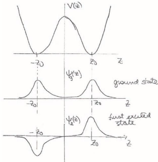
Figure 3: The potential  $V(z)$  experienced by the nitrogen atom. There are two classically stable positions  $\pm z_0$ . The ground state and (first) excited state wavefunctions  $\psi_g(z)$  and  $\psi_e(z)$  are sketched below the potential.
