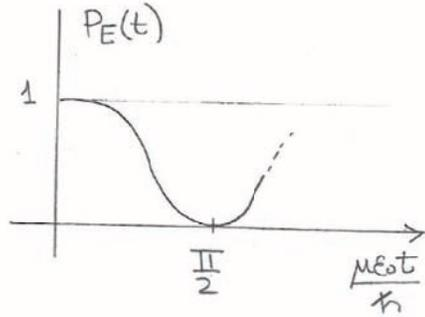
Figure 8: An ammonia molecule enters the resonant cavity at  $t = 0$  in the excited state  $|E\rangle$ . We show probability  $P_E(t)$  for the ammonia molecule to be in the excited  $|E\rangle$  at time  $t$ . If the molecule exits at a time  $T$  for which  $P_E(T) = 0$ , the molecule will be in the ground state  $|G\rangle$ , as desired.
