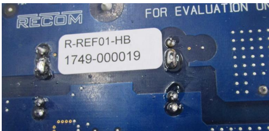
Figure 5: Create solder bridge
